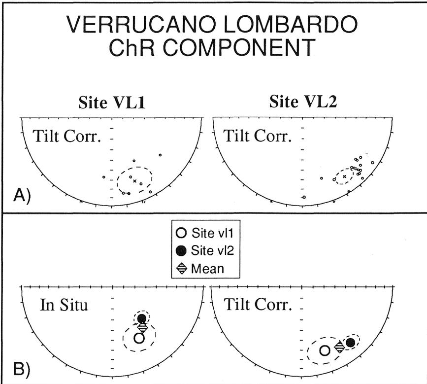
Fig. 6 - Stereographic projections of (A) the tilt corrected characteristic remanence detected in the Verrucano Lombardo Ss. sites, provided with the a95 cone of confidence around the mean and of (B) the mean direction of the characteristic remanence of each site before and after correction for tilting.
