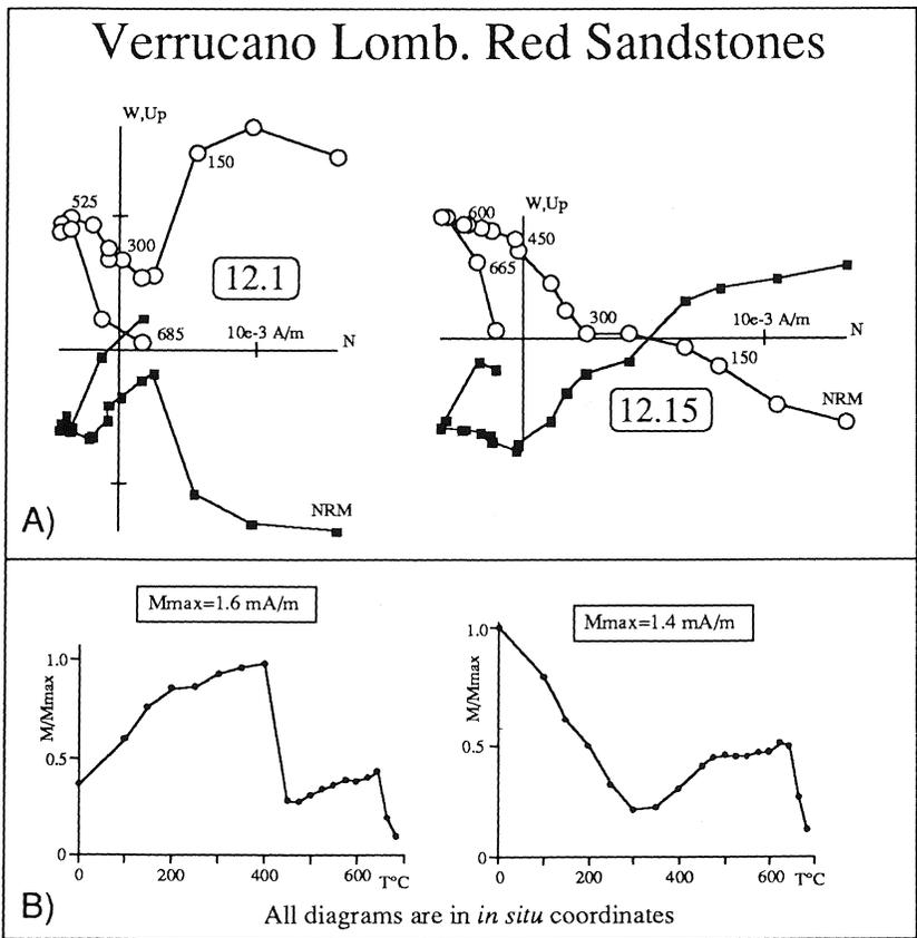
Fig. 4 - (A) Examples of orthogonal projections of thermal demagnetization data and (B) curves of thermal decay of Natural Remanent Magnetization (NRM) for two Verrucano Lombardo Ss. samples (site VL2). Solid squares are projections onto the horizontal plane, open circles onto the vertical plane. All diagrams are in *in situ* coordinates. See text for discussion.
